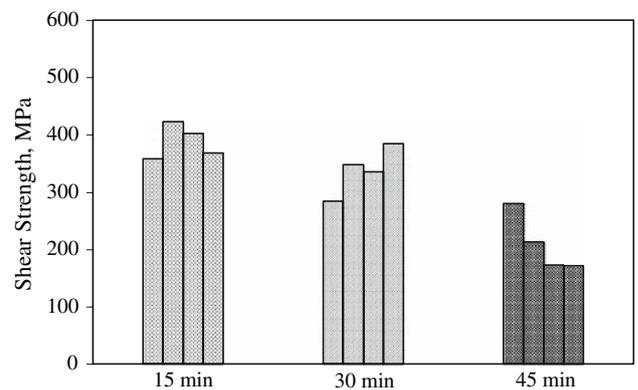
**Fig. 11** The effect of time on the joint performance for the bonds produced at 825 °C/5 MPa
