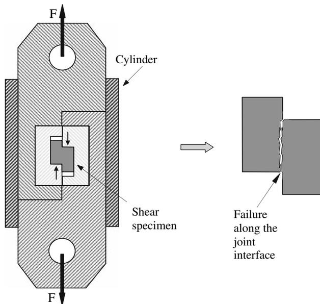
**Fig. 3** Schematic illustration of the shear testing
