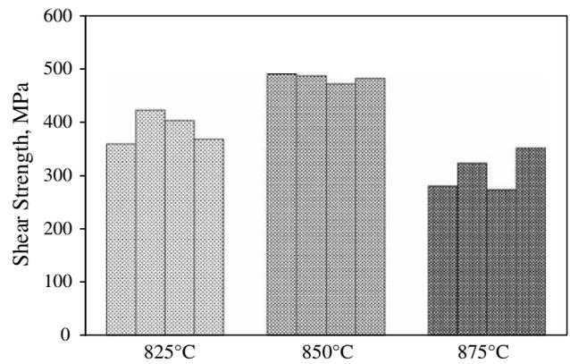
**Fig. 10** The effect of temperature on the joint performance for the bonds produced using a pressure of 5 MPa for 15 min
