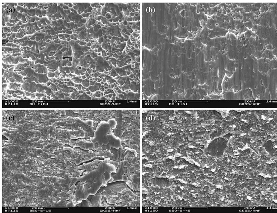
interface, i.e. 1.5–2  $\mu\text{m}$ . The increase of the thickness of this brittle phase beyond this critical value results in a degradation of joint performance. Thus, beyond the critical thickness of the brittle phase forming at the interface, the presence of brittle reaction product becomes more critical in affecting the bond strength. The highest shear strength value has been obtained with a bonding time of 15 min for a given set of other parameters.
